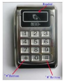
3.Encode management card:Read the master card again,then read another blank card.Then this blank card is encoded as management card.
